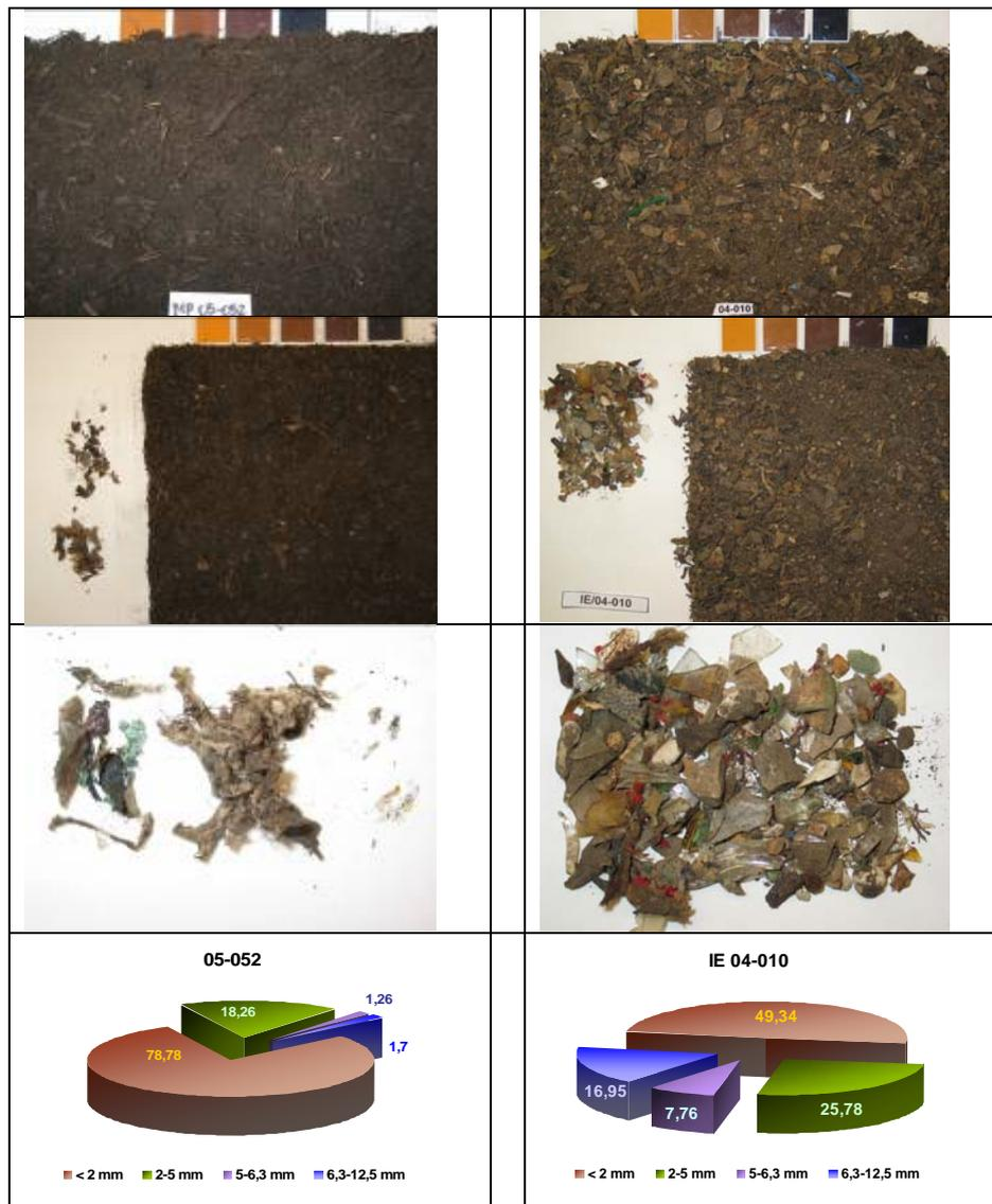
Figure 10.- Appearance, granulometry and content in impurities of two samples of municipal waste
